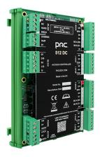
Complete with DIN mount for fitting in to PAC DIN mount cases (p/n 10031 and 10032)
